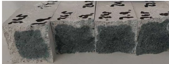
Fig.5.7 AAB mortar prisms after 28 days prepared at w/b of 0.345 prepared adding both 50 mM of \text{CaCl}_2 and 0.9 % of PCE (by weight of binder) stored in air.
